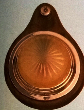
▼ A brass bulkhead light fixture, without its bulb. It was possibly used as a reading lamp over the cabin berth.
