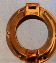
▲ A small round porthole, made from brass. It has a glass window which could be levered open for air.
